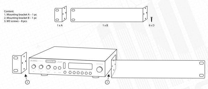
(1) Fix mounting brackets (A and B) to DMPA light amplifier and install equipment to the 19" rack.
