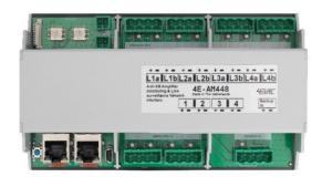
Each amplifier channel is split internally into 2 loudspeaker circuits: A and B.
